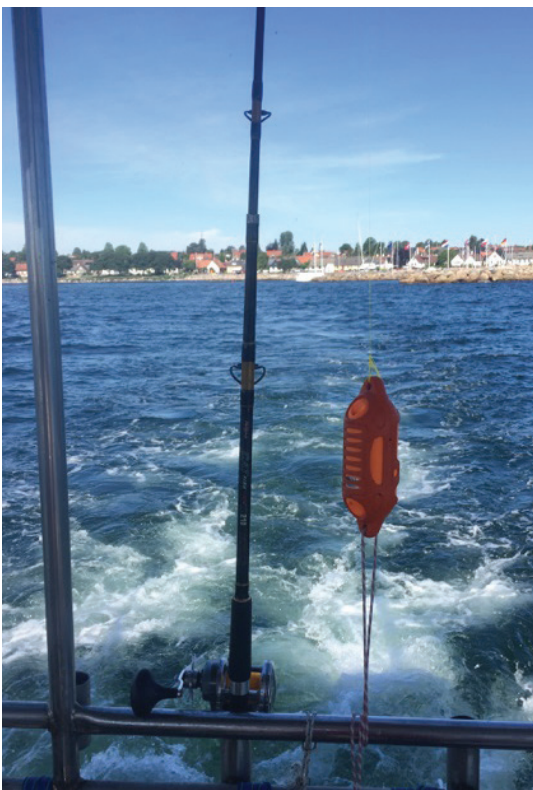
CastAway CTD hooked to fishing rod ready to collect water column profiles of Salinity and Temperature
