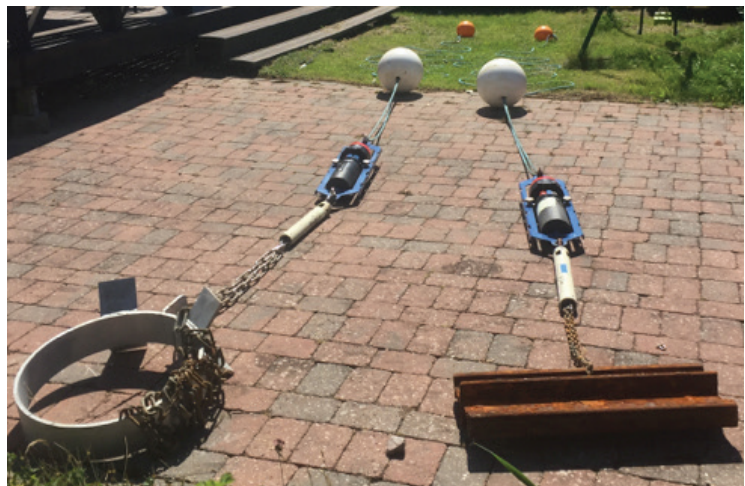
RDCP mooring systems.
