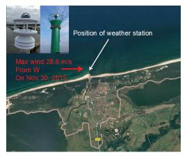
Fig. 2: Meteorological station in Leba (Polish N coast) is placed on top a lighthouse and consists of a <u>SmartGuard</u> logger, a GSM modem and a <u>Gill GMX 600</u> weather sensor. A similar system is installed in <u>Gdynia</u> it is on-line and serves also for navigation aid.
